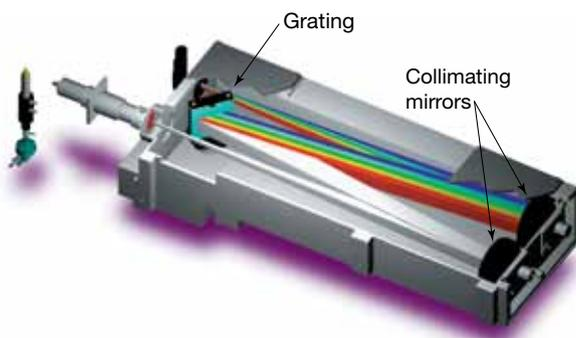
The large surface area of the grating allows for collecting more light and the illumination of more grooves, thus improving resolution. The JY 2000-2 utilizes a classic Czerny-Turner design with only two reflective surfaces in addition to the grating.
